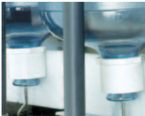
Bottle holding mechanism ensures that bottles are protected during wash cycles.
