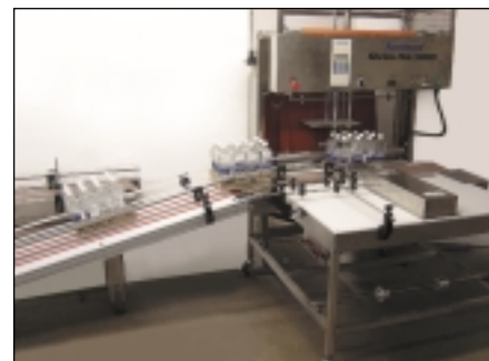
Bottles entering Norland's Shrink- Pak™ 5000 from CasePak 5000's optional lift conveyor for automatic wrapping
