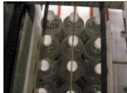
Bottle support knives ensure proper alignment
