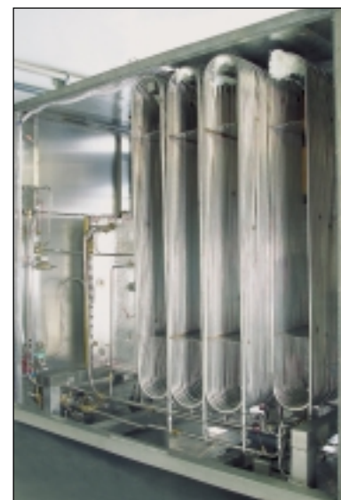
Tube-in-tube heat exchangers provide highly efficient heat transfer to incoming feed-water for power consumption per gallon as low as .085 Kw/H.
