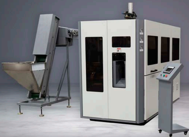
Blow Molder (Produces Plastic Bottles)
