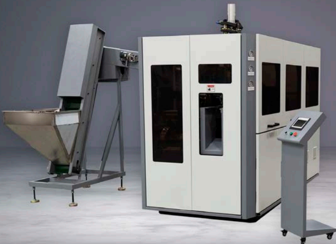
Blow Molder (Produces Plastic Bottles)
